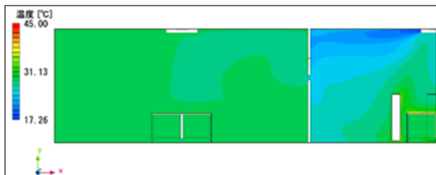
Figure 17. Air temperature of Case 5. The target zone's average air temperature was 26.7°C, while the average air temperature in the non-target zones was 28.5°C, respectively
